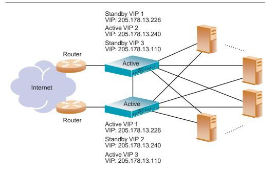
Figure 11-4 Active-Standby Redundancy
